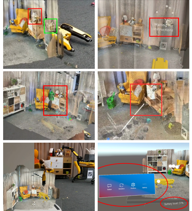
Fig. 3: HoloLens Interface. The above figures show various aspects of the visual interface on HoloLens. Labeling images with number left to right, and top to bottom we have: on the first image bounding boxes displaying movable objects following ”show items” voice command, the following image shows how robot status is displayed during manipulation. Images four and five display user manipulating watering can and a drawer. On the fifth and sixth images we can see virtual representation of the robot and menu containing battery percentage and additional status information.
