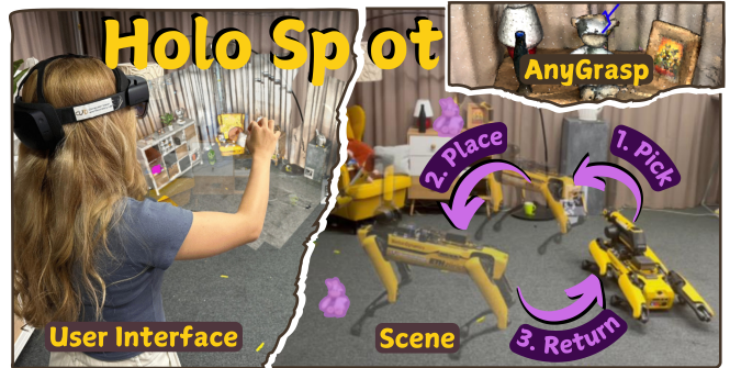
Fig. 1: Visualization of Our System. Left: A user wearing a HoloLens to interact with a holographic representation of the environment. Right: Robot pick-and-place sequence of actions. Top: Optimal grasp selection with AnyGrasp.
